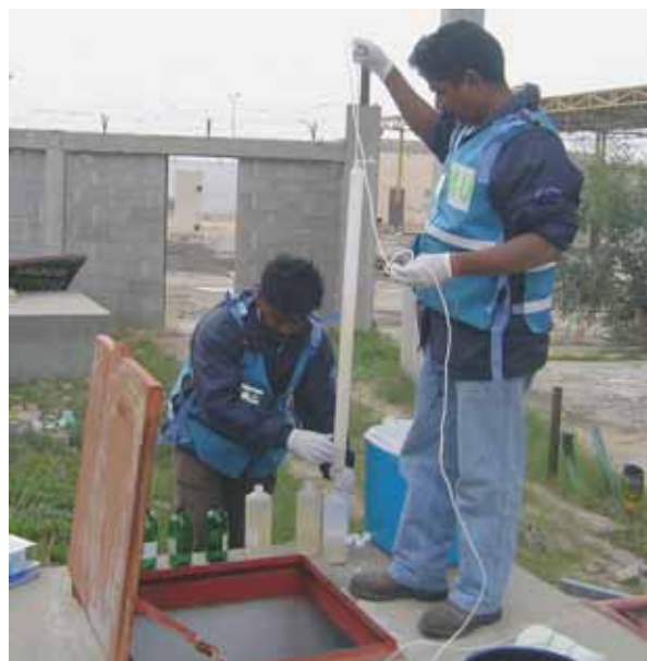
In some places disposable bailers were used to collect water samples
