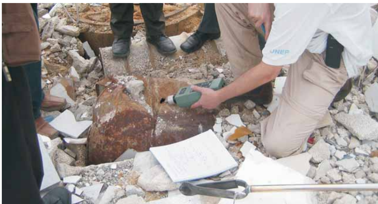
Sampling in the field using hand-held portable equipment
