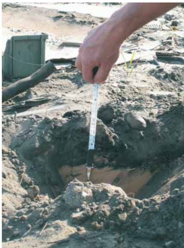
The maximum depth of the impacted "burnt" zone at location A was 10 centimeters
