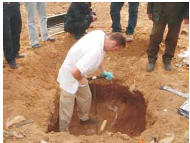
UNEP expert collecting a core sample from an excavation pit
